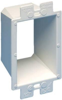
Arlington Industries (AI) manufactures these nifty box extenders which will extend the face of a device or junction box up to 1-1/2”, deliver a maximum two hour fire rating, and can be installed without having to disconnect the wires from the outlets or other fixtures in order to install them (just make sure the power is turned off). These box extenders are available in various gangs for walls as well as ceilings.
